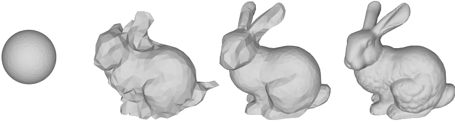
Figure 4.4: Our method reconstructing the Stanford Bunny starting from a sphere. From left to right: Initial mesh (sphere), after 50 iterations, after 750 iterations, and the converged result. The final reconstruction has 13 780 vertices and has a symmetric volume difference of 0.30%, when compared to the ground truth. Figure from Contribution F .
