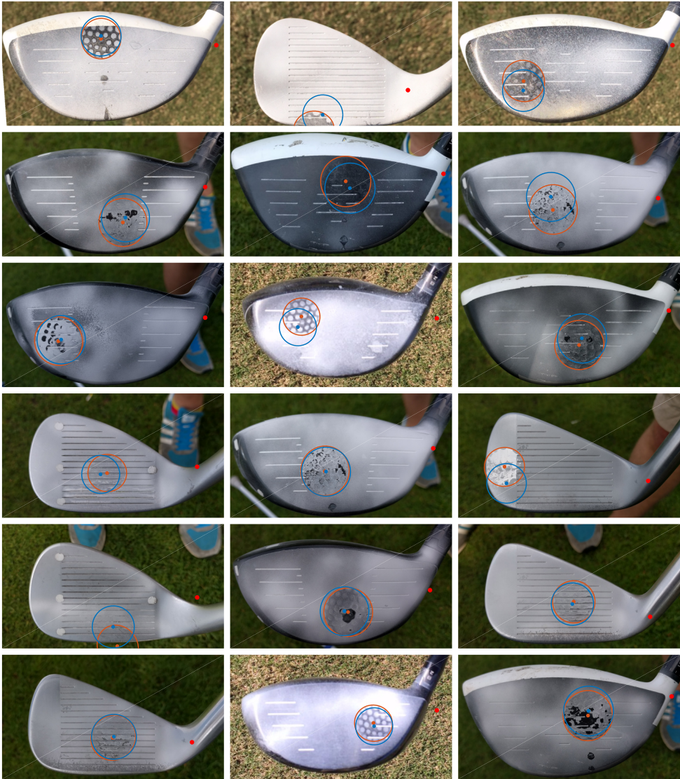
Figure 5.24: Random selection of predicted impact locations. Red circles are the annotated positions and blue circles are the predicted ones. The red dot is the used anchor point.
