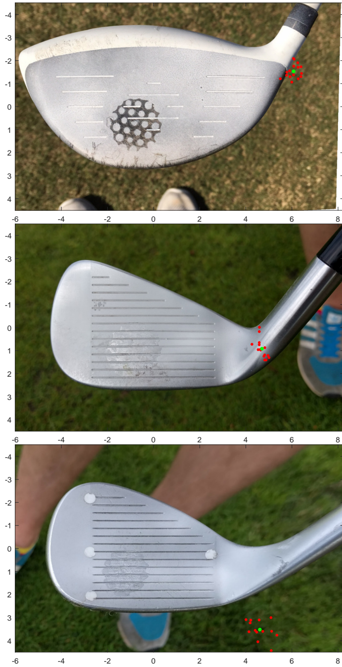
Figure 5.20: Computed \mathbf{v}_{ap,i} s shown on top of the corresponding club. The red points are the anchor point clouds, while the green points are the means. From top to bottom: DS1 Driver 1, DS2z Iron 2 and DS2n Wedge 2. The method is smoothing spline and M3. Units are cm.
