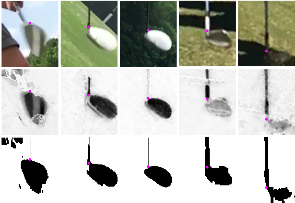
Figure 5.9: Images showing the result of our club head segmentation with their respective detected anchor points. Top row: color image, middle row: difference image, bottom row: segmentation.
