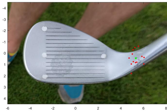
Figure 5.21: Computed \mathbf{v}_{ap,i} s shown on top DS2n Wedge 2 in red. The green point is the mean. Units are cm.
