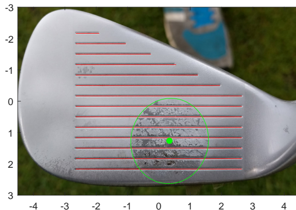
Figure 3.7: Ground truth example, where the image has been transformed using the homography. Red is standard lines, green is annotated impact ball. Axes are in cm.
