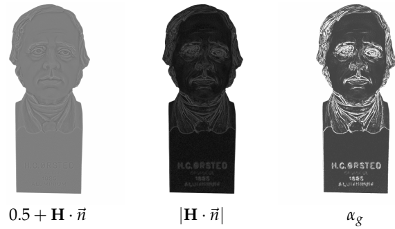
Fig. 3. Model of spatially varying roughness \alpha_g for an aluminium bust that has from time to time been subjected to hand polishing. We use the dot product of the mean curvature normal \mathbf{H} and the surface normal \vec{n} . The model correctly marks eyes, hair, nostrils, and engraved letters as rough, but also incorrectly marks edges along the box-like base of the bust as being very rough.
